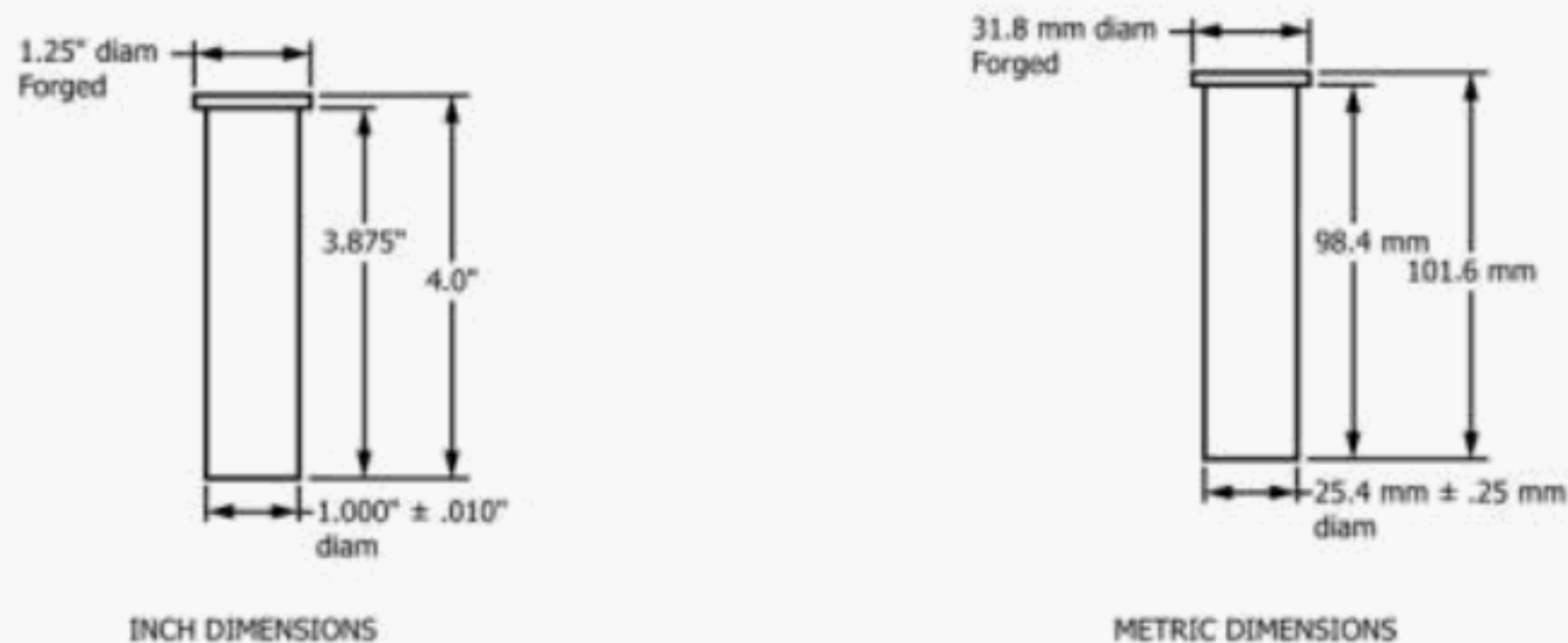
FIG. 2 Preferred Test Specimen
